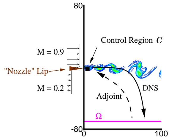
**Fig. 1** Mixing layer control schematic. The line  $\Omega$  is the support of the noise metric to be minimized. The small black box  $C$  near the “nozzle” lip shows the support of the control. Arrows indicate the DNS solution (forward in time) and the adjoint solution (backward in time), which provide the sensitivity data.
