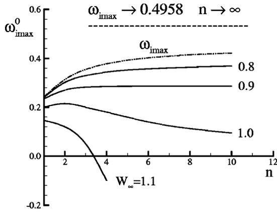
FIG. 3. The variation of maximum absolute growth rate as azimuthal wave number. The dash line shows the maximum temporal growth rate.
