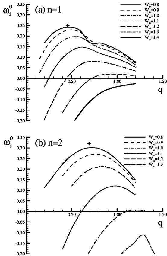
FIG. 1. The variation of absolute growth rate  $\omega_i^0$ . The plus (+) symbol indicates the maximum temporal growth rate  $\omega_{i\max}^0$  (a)  $n=1$ ; (b)  $n=2$ .
