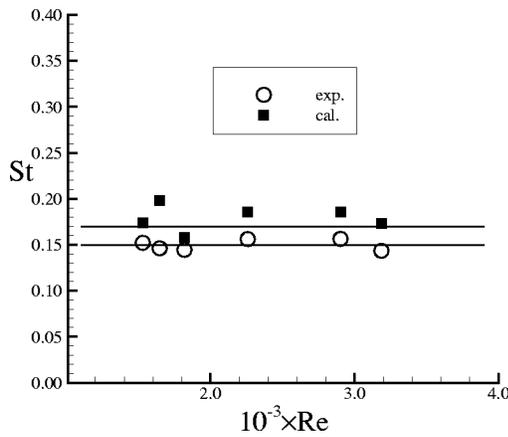
FIG. 14. Dominant Strouhal numbers in a breakdown bubble.  $St=0.171$ : theoretical prediction.  $St=0.15$ : average of measured values (Ref. 30).
