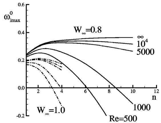
FIG. 7. Viscous effect on absolute growth rate with  $W_\infty = 0.8$  (solid lines) and 1.0 (broken lines).
