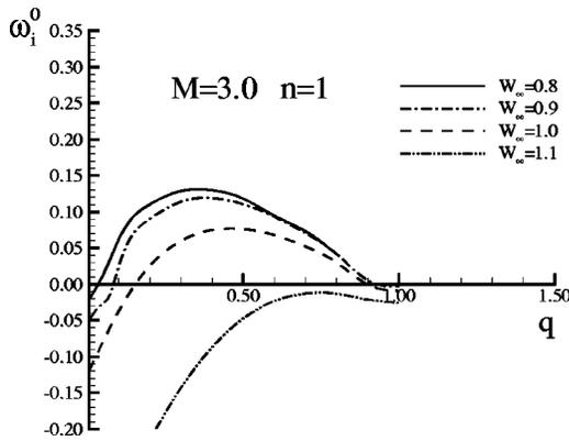
FIG. 9. Effect of axial velocity deficit on  $\omega_i^0$  for  $M=3.0$  and  $n=1$ .
