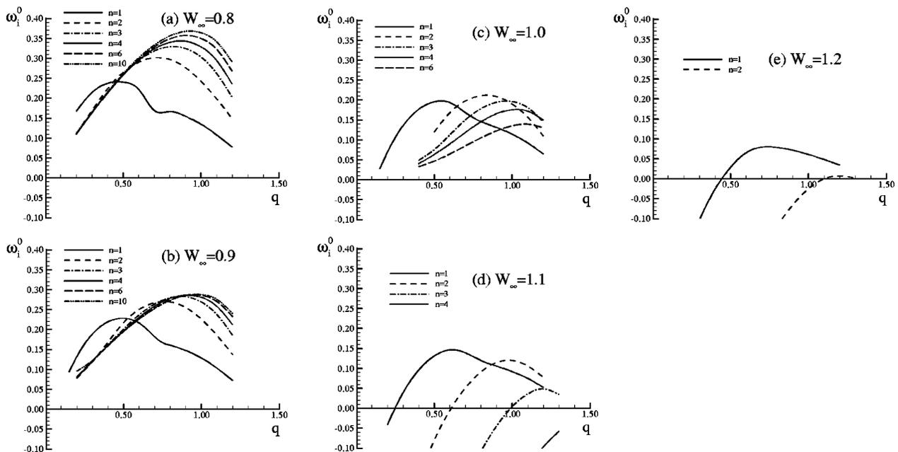
FIG. 2. The variation of absolute growth rate  $\omega_i^0$  as  $q$  for different azimuthal wave numbers. (a)  $W_\infty=0.8$ ; (b)  $W_\infty=0.9$ ; (c)  $W_\infty=1.0$ ; (d)  $W_\infty=1.1$ ; (e)  $W_\infty=1.2$ .
