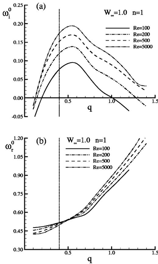
FIG. 5. The variation of (a) absolute growth rate  $\omega_i^0$  and (b) absolute frequency  $\omega_r^0$  as  $q$  for different Reynolds numbers.  $W_\infty = 1.0$ ,  $n = 1$ .
