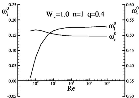
FIG. 6. Effect of viscosity on  $\omega_i^0$  and  $\omega_r^0$ .  $W_\infty = 1.0$ ,  $q = 0.4$ ,  $n = 1$ .
