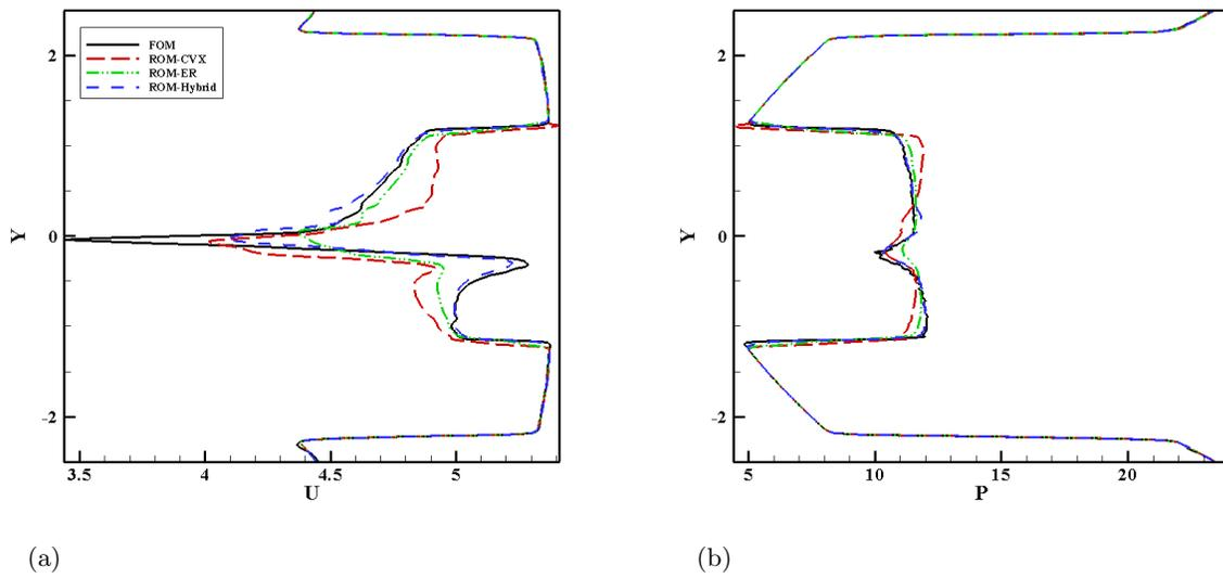
Figure 4: Profiles of a) horizontal component of velocity and b) pressure, reconstructed by linearized ROMs with 16 modes compared against the FOM.
