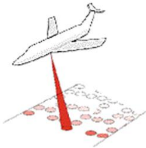
Figure 1: Airborne LIDAR randomly emitting pulses across a region.
