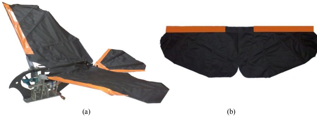
Figure 6. (a) Thunder I FWMAV and (b) wing of the Thunder I FWMAV.
