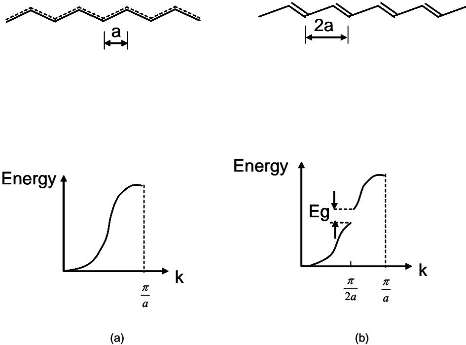
Fig 2.2 Process of transition from (a) metallic state to (b) non-metallic state by dimerization.
