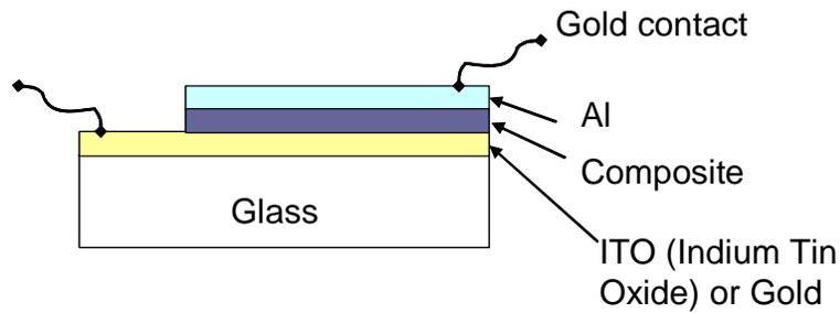
*Fig. 6.1 Sandwich cell for device testing*
