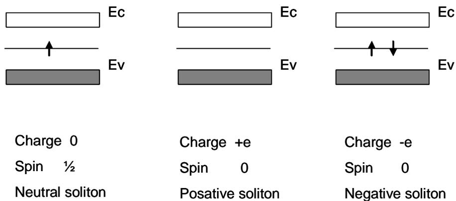
*Fig 2.5 Charge and spin combinations for differently charged solitons.*
