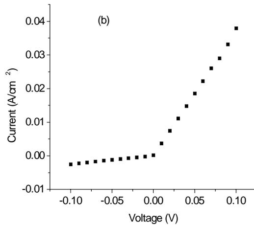
Fig 6.2 J-V plot of (a) Al/PmPV/Au cell; and (b) Al/PmPV-gold nanocomposite/Au cell
