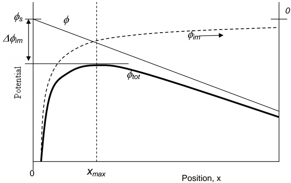
Fig 2.10 Schematic of barrier lowering caused by the image force effect.
