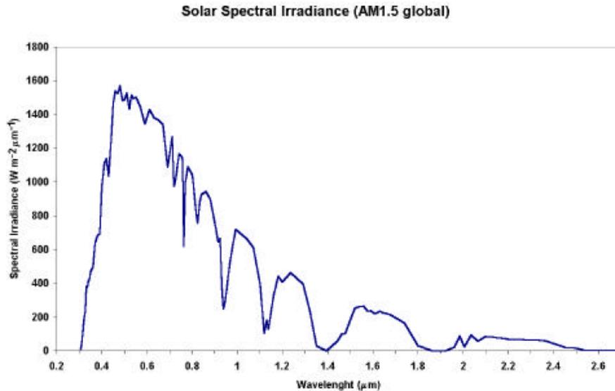
*Fig 3.2 The standard AM1.5 global solar spectrum*
