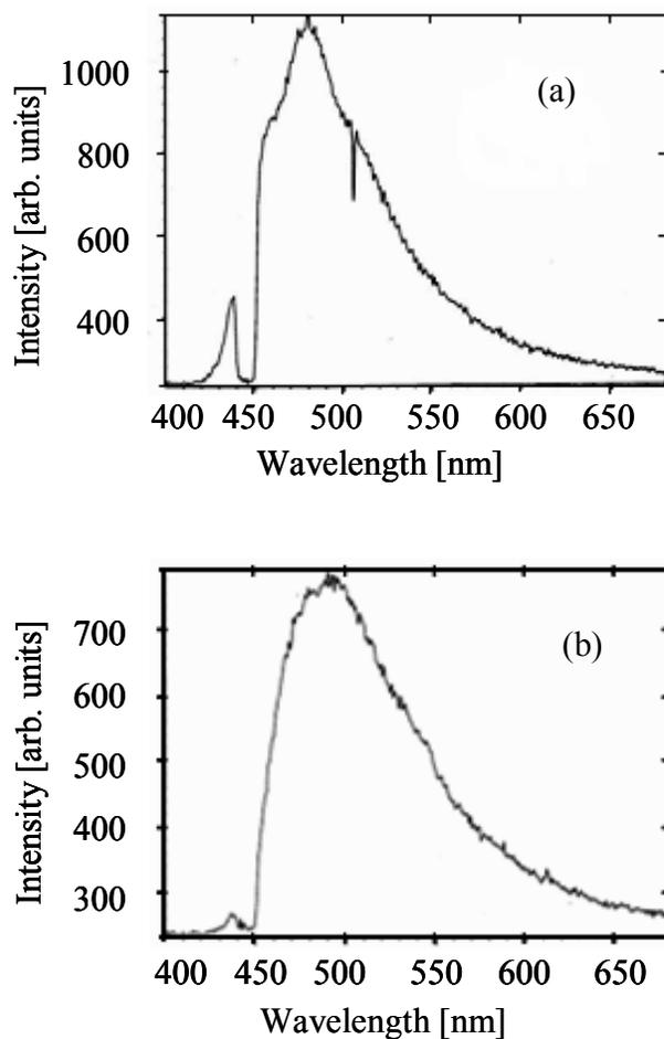
*Fig 4.4 Near field fluorescence spectra of PmPV (a) and PmPV- C<sub>60</sub> composite (b)*
