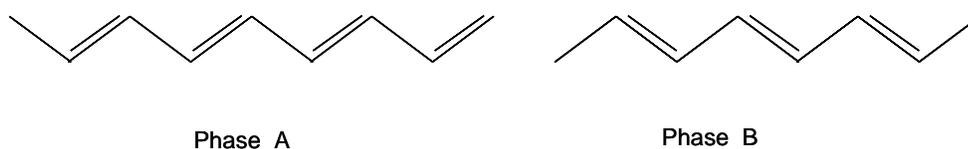
*Fig 2.3 Degenerate ground states of trans-polyacetylene*
