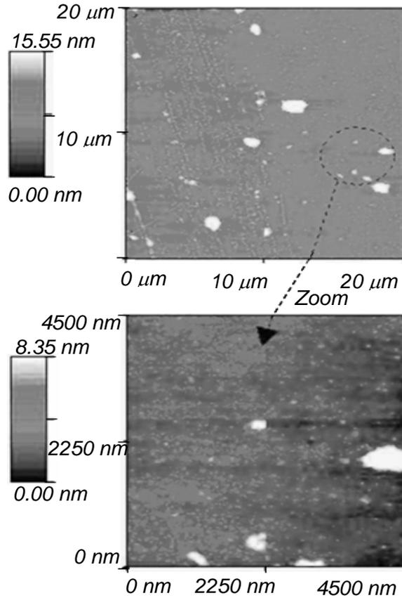
*Fig 4.3 Atomic Force Microscopy topographic images of PmPV/ $C_{60}$  nanocomposite.*
