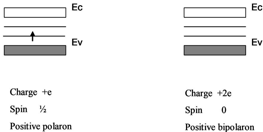
Fig 2.8 Energy band diagrams showing charged states of a non-degenerate ground state polymers.
