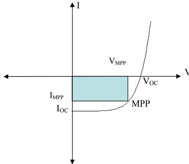
*Fig 3.1 Typical shape of the current–voltage curve of a photovoltaic cell showing the open circuit voltage  $V_{OC}$ , short circuit current  $I_{SC}$ , the maximum power point MPP, and the current and voltage at the MPP;  $I_{MPP}, V_{MPP}$*
