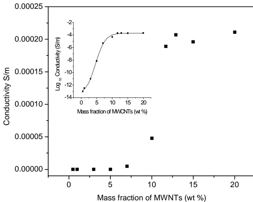
*Fig 5.4 A plot of DC conductivity of pristine MWCNT-polystyrene blend as a function of mass fraction of pristine MWCNTs in the blend. Inset: a semilogarithmic plot of pristine MWCNT-polystyrene blend conductivity as a function of mass fraction of pristine MWCNT in the blend. The solid line represents a curve fit using (5.1)*
