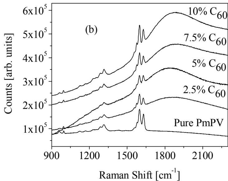
Fig 4.5 Raman Spectra of PmPV/C<sub>60</sub> composite for 785 (a) and 514 (b) laser lines.
