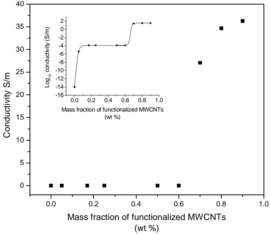
Fig 5.3 A plot of DC conductivity of covalently linked MWCNT-polystyrene composite as a function of mass fraction of functionalized MWCNTs in the composite. Inset: a semilogarithmic plot of covalently linked MWCNT-polystyrene composite conductivity as a function of mass fraction of MWCNT in the composite.
