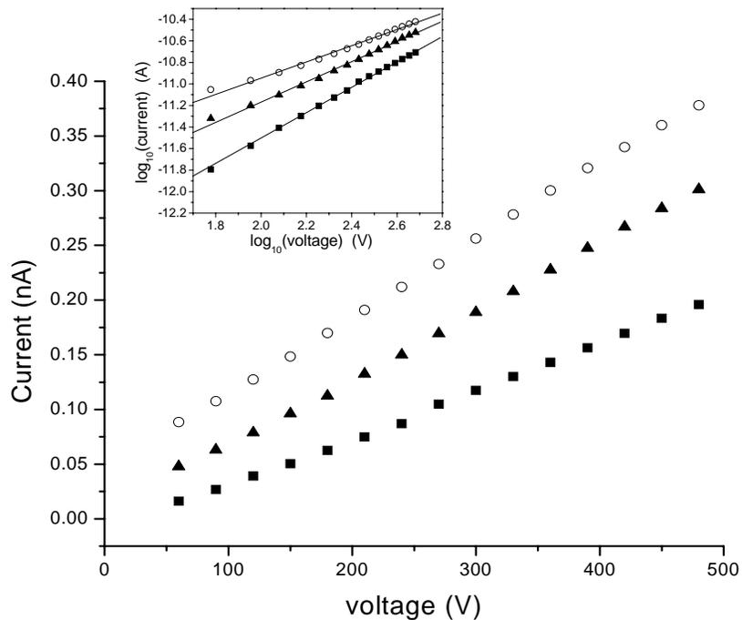
*Fig 5.5 A plot of current vs voltage for pure PmPV (■), 15% wt/wt concentration of gold particles in PmPV (▲) and 30% wt/wt gold particles in PmPV(○). Inset: Corresponding logarithmic current – voltage characteristic.*
