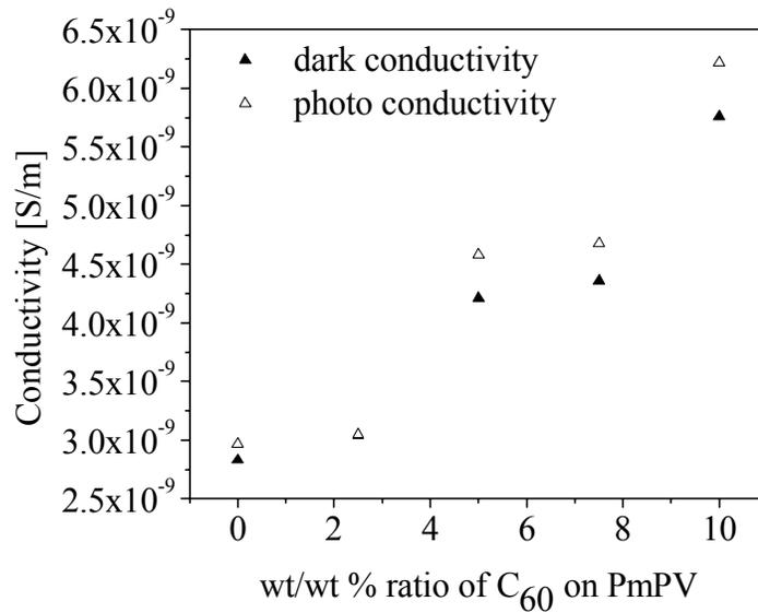
Fig 5.2 Dark and photo conductivity of polymer/C<sub>60</sub> composite for different concentrations of C<sub>60</sub>
