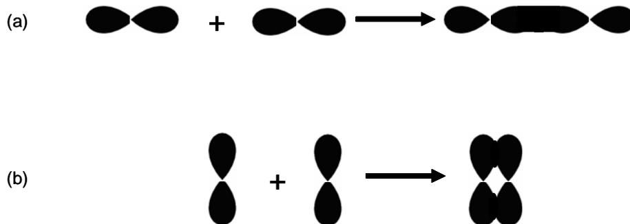
*Fig 2.1 (a) Overlap of two p atomic orbitals to give a bonding  $\sigma$  MO. (b) Overlap of two p atomic orbitals to give a bonding  $\pi$  MO.*
