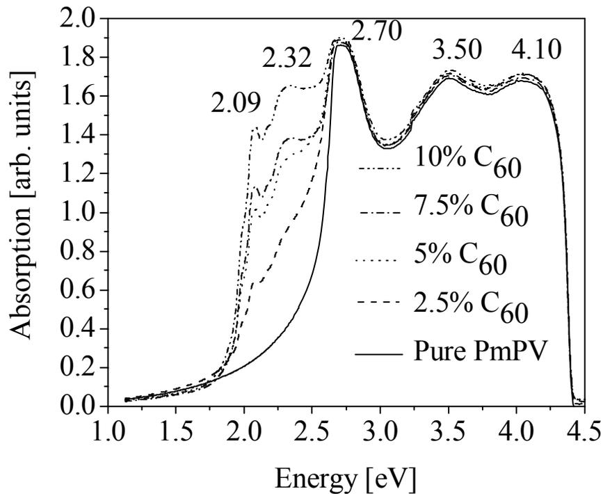
*Fig 4.2 UV-Visible spectra PmPV/ $C_{60}$  nanocomposite for different concentrations of  $C_{60}$ .*
