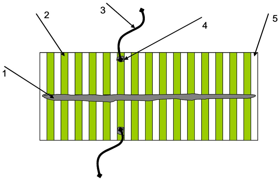
*Fig 5.1 shows a typical conductivity measurement sample prepared on a glass substrate.*
