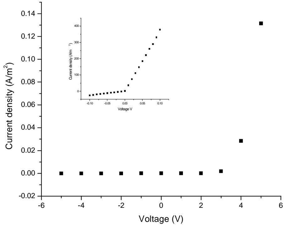
*Fig 6.3 J-V plot of Al/PmPV/Gold sandwich cell with inset of Al/PmPV-Au composite/Gold cell.*
